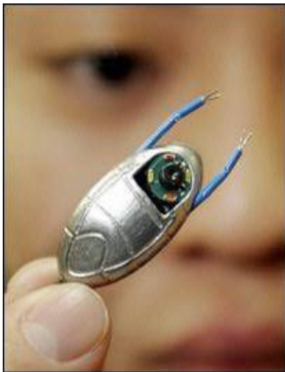
Micro medical Robot aims to minimize the need for surgery, this surgical micro robot can affix diverse kind of medical devices such as micro camera, micro manipulators, various sensors and drug delivery injector.
