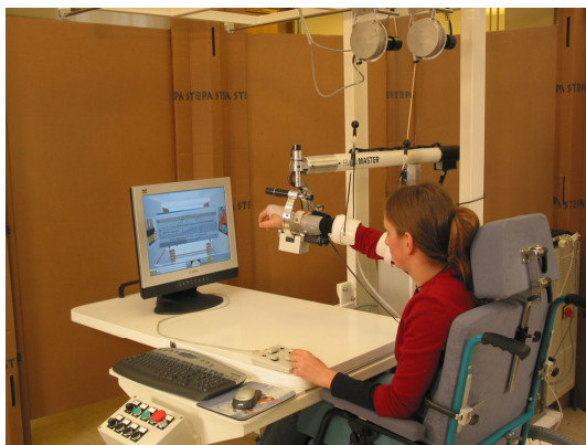
The Gentle/S system was developed and tested in an EC funded project. It aims at offering force feedback guidance in moving the affected arm in order to effectively train its control.
