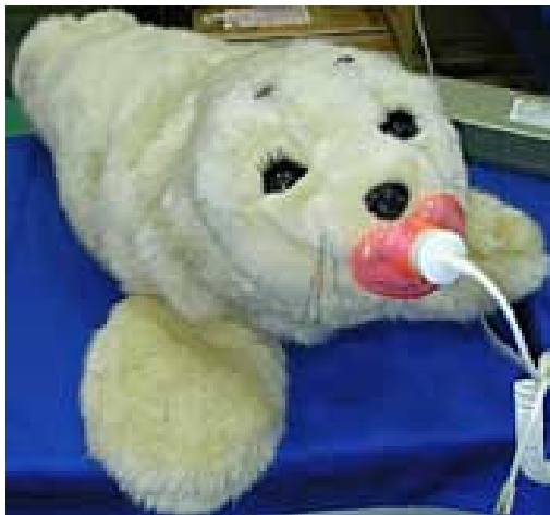
Covered in soft white antibacterial fur, Paro's artificial intelligence means it can mimic animal behavior and over time, develop its own character.
