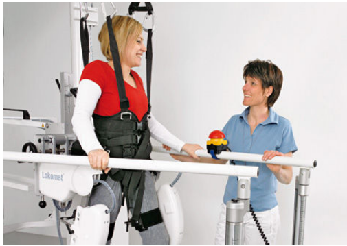
Hocoma's Locomat is a system designed to support the patient in restoring gait patterns while taking away the body weight on the patients legs.
