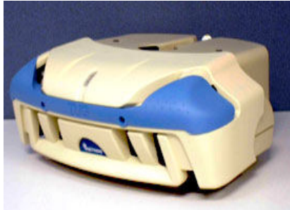
The TUG system transports a variety of hospital carts. It automates and tracks the delivery of goods in hospitals.
