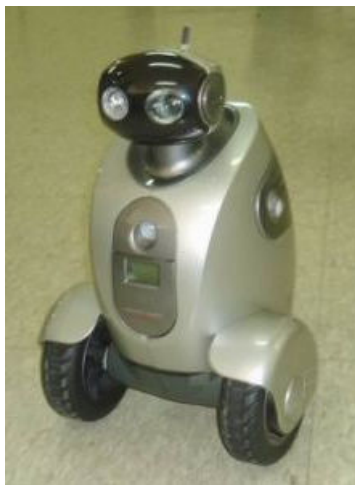
The Mir-H platform provides a mobile system able to monitor safety and activity at home.
