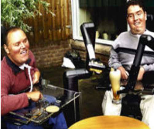
ARM manipulator arm by Exact Dynamics BV (the Netherlands). Robot manipulator consisting of a mechatronic robot arm mounted on an electrical wheelchair controlled by a joystick and button device mounted on the armchair.
