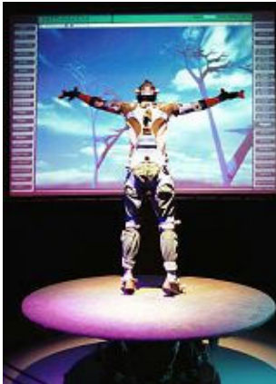
Caren consists of a force platform and a virtual environment able to map human movement in controlled conditions
